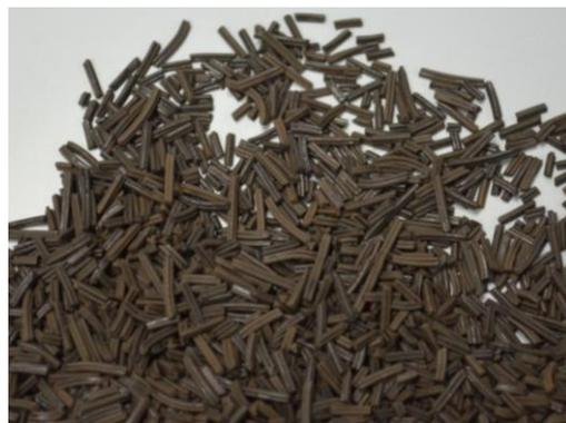
Three-way catalyst for hydrotreatment of vacuum gasoil
