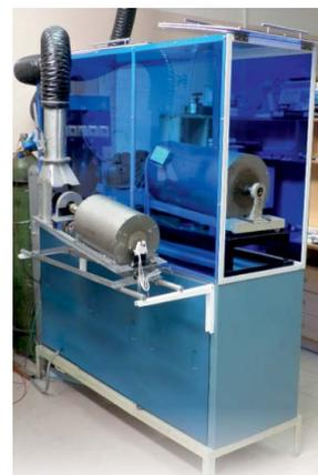
A pilot plant (up to 5 kg MWCNT/day capacity) with fluidized catalyst bed has been put into operation.
